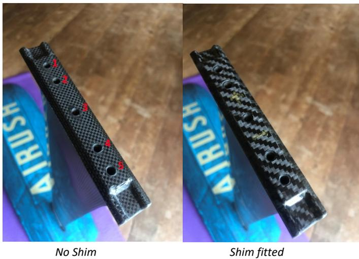
Place and hold the glider over the shim (it should seat nicely on the contact face). Place a small amount of the supplied TefGel on the lower portion of each of the 5 M5 BUMAX 88 fastener (15 provided) and insert into the glider holes.
