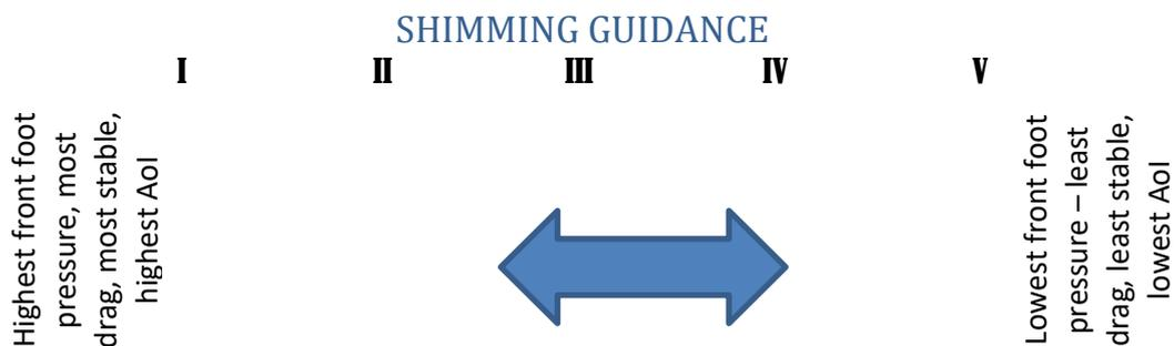
*For the first ride, we suggest shim I or II to initially get the feel for the foil, and light to moderate wind. After getting used to the foil and front foot pressure, you can go to the more advanced shims and ride in higher wind conditions.*
