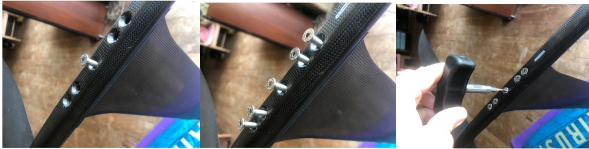
Again, starting with the fastener 3 position, and using the tool with 5Nm marked on it, tighten 1/4 turn, repeat with fastener 2, then fastener 4, then fastener 1 and lastly fastener 5.
